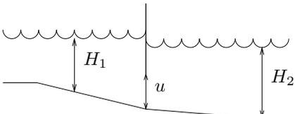
Here,  $H_i$  is the height of water in the  $i$ -th part of the canal;  $g, \nu$  and  $\alpha_i$  are as above. The system is controlled through  $u$ , which is the height of the opening in the gate.
